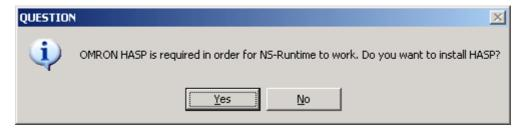
When installing the NS-Runtime in the NSA Series, a message confirming the HASP driver installation will be displayed. Click the **OK** Button. For information on HASP driver installation, refer to 2-2-2 Installing the HASP Driver.
