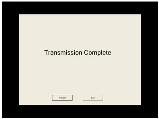
13. Click the **Restart** button to close the transfer screen and to end the NS-Runtime. Click the **Exit** button to close the transfer screen.
